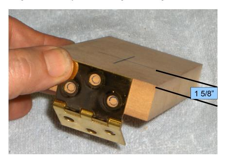
First, mark a spot 1 5/8" from one of the ends and halfway between the long sides. Then hold a hinge against the same end (centered side-to-side, with its edge aligned to the face of the MDF) and mark the three hole locations.
