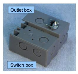
Once the boxes are glued together, mount the cord clamp in the remaining knockout hole. Drill out the appropriate mounting holes, using the "pre-molded" features inside the rear surface of the box(es). For corner installation on an MDF Rose Engine, these are the ones on the switch box - the one without the cord clamp.
