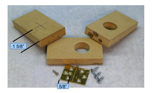
Once you have the switch operator and hinge drilled and the operator smoothed, they can be assembled to each other, masked and painted. If you use spray paint, be sure you've carefully masked the barrel section of the hinge, so the paint doesn't get in and gum it up. I like to use red paint, as in "Hit red to stop." If you want to (later on), you can put some green electrical tape on the upper half of the Decora switch - "Green for go."
