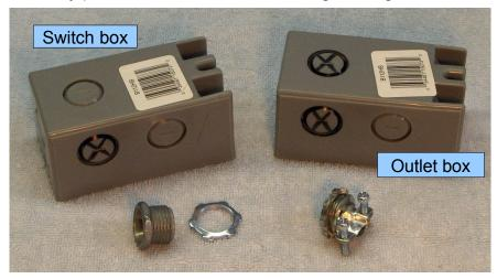
Assuming you want to mount the switch assembly at the right front of an MDF Rose Engine, "surrounding" the corner as shown in the first photo, remove two of the knockouts (marked "X") from one box and one from the other. You can of course vary the configuration to fit your Rose Engine; remove whatever knockouts are appropriate. What you'll need, regardless of configuration, is a through-hole between the boxes and a power cord entry hole in one of them.
