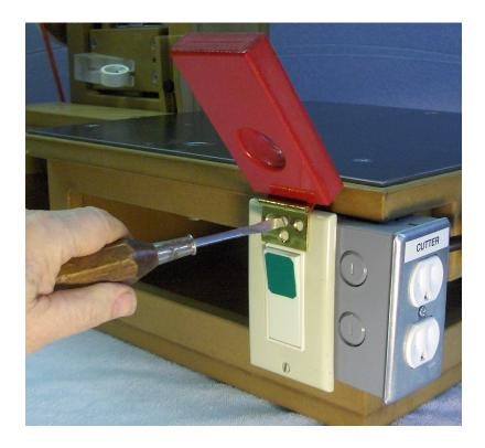
Verify that the operator swings freely and that its lower section positively shuts the switch off when any part of the operator's front surface is pressed. If necessary, add a small self-stick felt bumper about an inch from the bottom of the operator.
