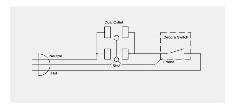
Along with specifying the cord length, you'll want to ask your electrician to be sure to mount the Decora switch correctly. It's very important that that the end marked "TOP" is indeed at the top. Otherwise, the on/off functioning of the switch will be incorrect!
