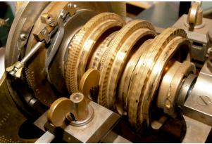
Notice the differences between the rosettes characteristic of a woodturning rose engine on the left, and the more subdued and higher-count patterns of those on a typical metal working rose engine on the right.
