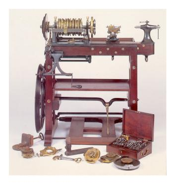
Engine turning encompasses rose engine work. A rose engine differs from other lathes in many ways, but the biggest difference is that the headstock is not stationary. The headstock is hinged, allowing it to pivot back and forth, called rocking. By controlling this rocking motion with a roset-te—a cam-like disk—you can cut countless patterns.
