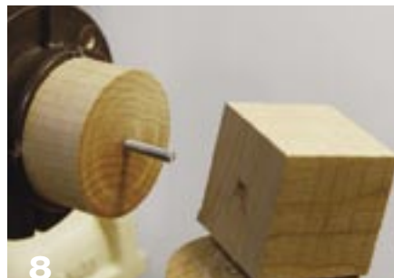
8 Drill the knob blank to mount on the wasteblock. Harden the wood threads with CA glue.
