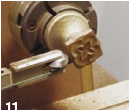
11 Make the decorative cuts on the face of the knob. Notice how phasing was added to position the points of one pattern in the rounded lobes of another.
