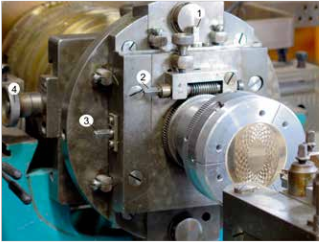
Figure 23 Various adjustments to the double eccentric and elliptical chucks
