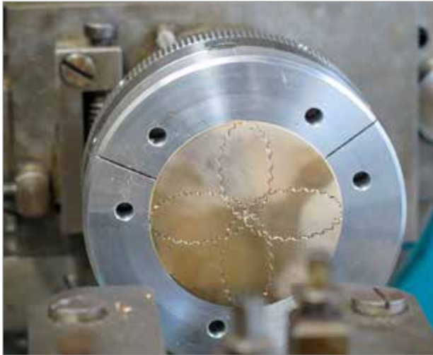
Figure 24 This example shows the effect of off-center turning and rotational adjustment. The rotational adjustment was indexed four times each at 90 degrees.
