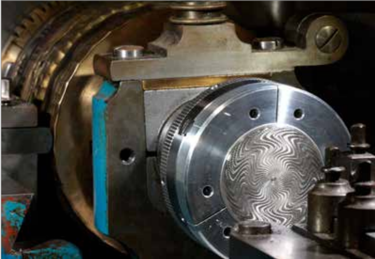
Figure 34 Work completed from outside towards center
